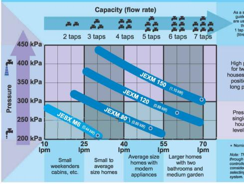
As a simple selection guide, tap symbols are used to represent the flow rate. 1 tap = 10 to 12 lpm (litres per minute)
